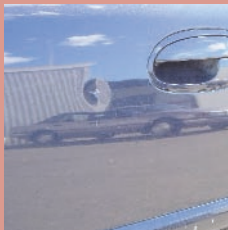
Dents of more than 20mm in diameter or paint surface penetration
